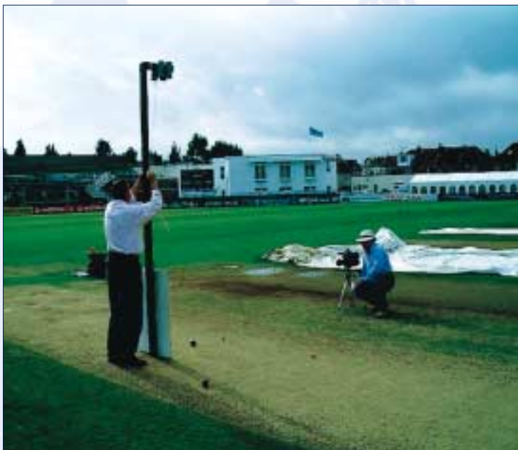
The three metre ball drop test.
